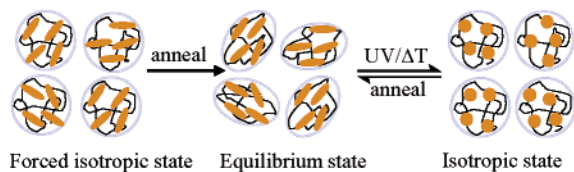
Figure 4. Thermal and UV shape shifting in azo-LCE disks.
